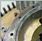
Pitting on bearing
